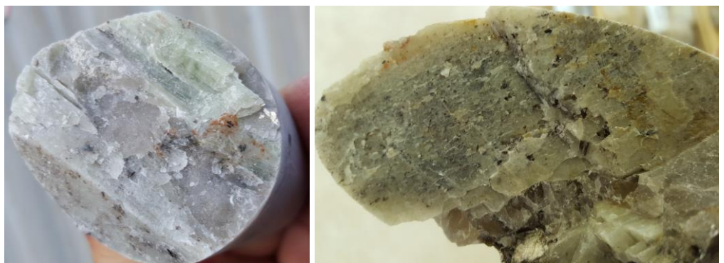
Figure 1. Various forms of Spodumene crystals identified in the drill core samples from the Seymour Lake project.
