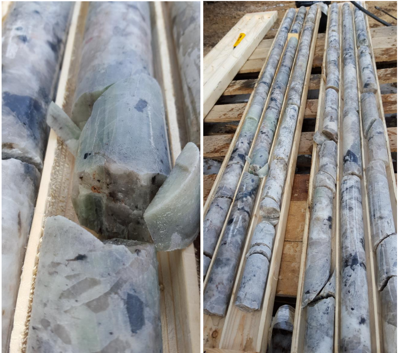
Figure 2. Drill Core from the Seymour Lake project showing multiple intersections of spodumene mineralisation in the pegmatite structures.
